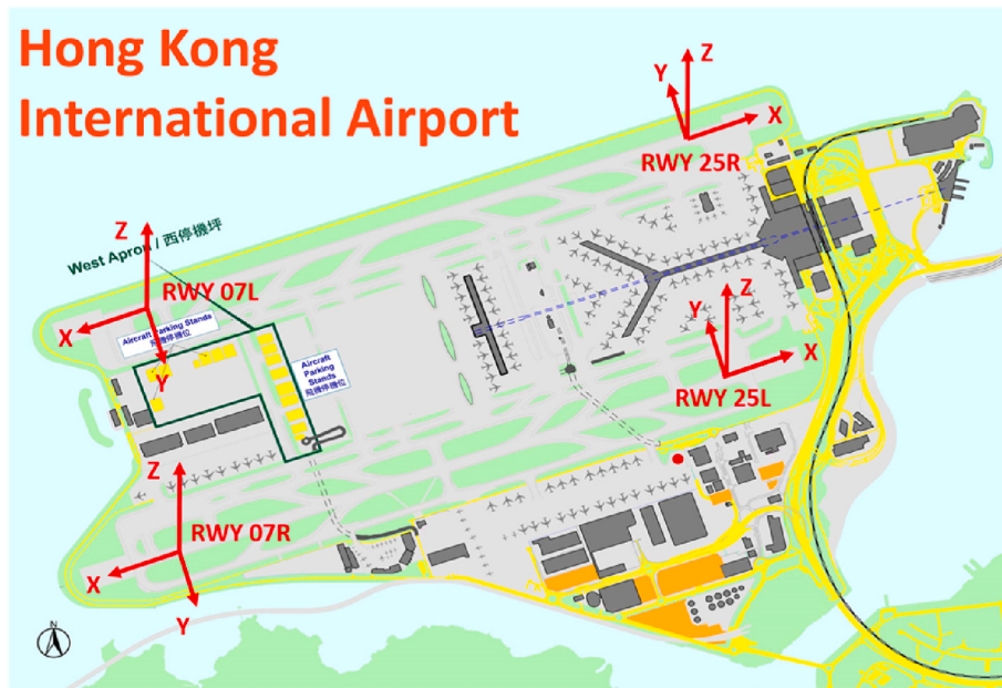
Fig. 11. Coordinate system transformation for HKIA.
